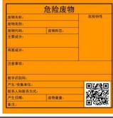
The label is orange with a black border. It has a header '危险废物' (Hazardous Waste) and a QR code in the bottom right corner. There are several fields for information, including '废物名称:' (Waste Name), '废物代码:' (Waste Code), '危险特性:' (Hazardous Characteristics), '数量/重量:' (Quantity/Weight), '包装形式:' (Packaging Form), '贮存日期:' (Storage Date), '责任人:' (Responsible Person), and '联系电话:' (Contact Number). | / |
